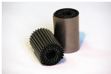
Figure 1 The monolith blocks produced from the FeCrAl foil and prepared for deposition of oxide coating by the EPD method.
